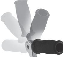
The rocking handle of the power tool can be secured in five different positions. Using different angles of the forward hand grip eases work load in different working positions. For right- and left-handed users. To tilt the handle, unscrew the handle for a few turns, bring the handle in the desired position, lock the handle by screwing it snug.
